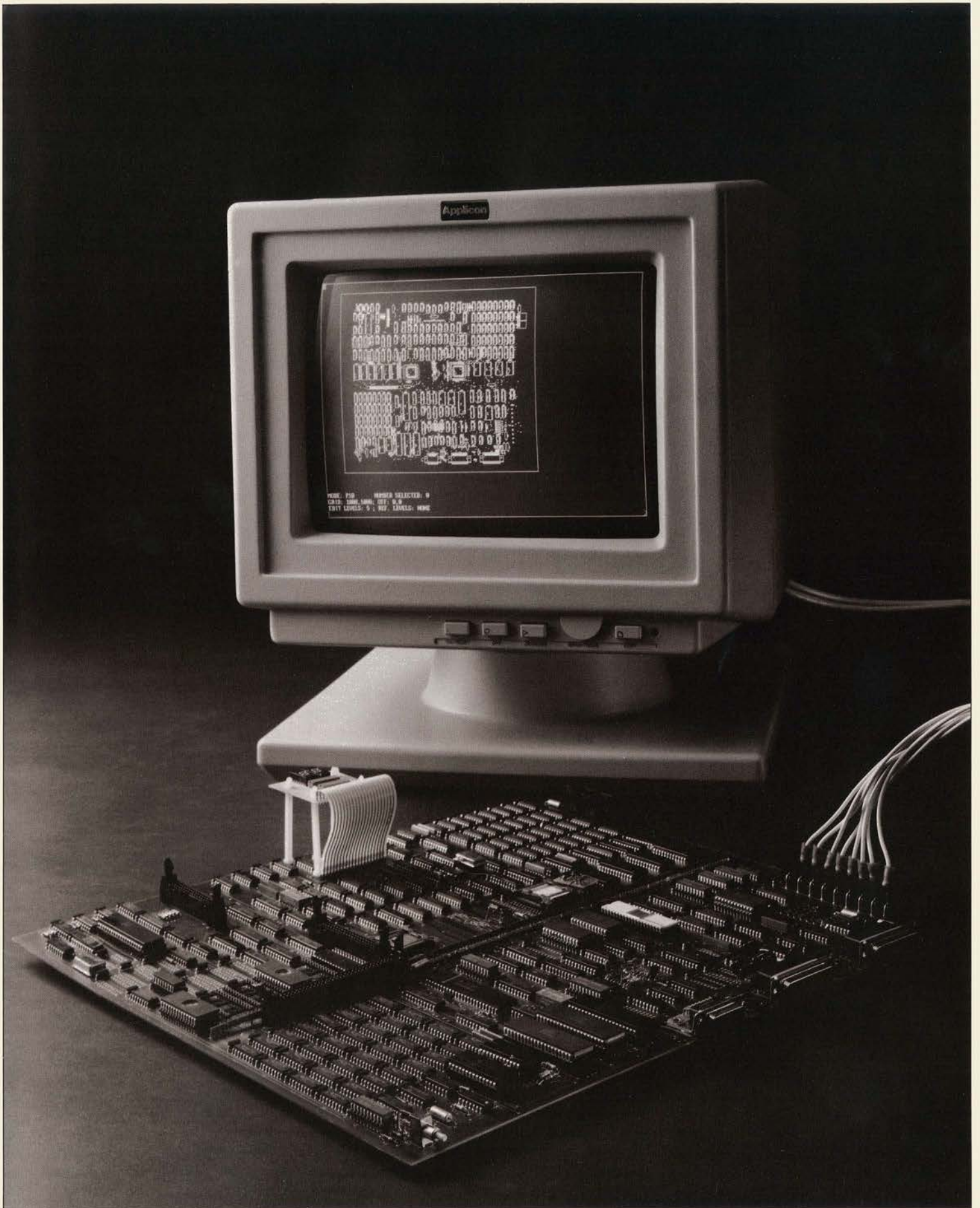
An important use of Applicon Computer Aided Design is laying out printed-circuit boards.
