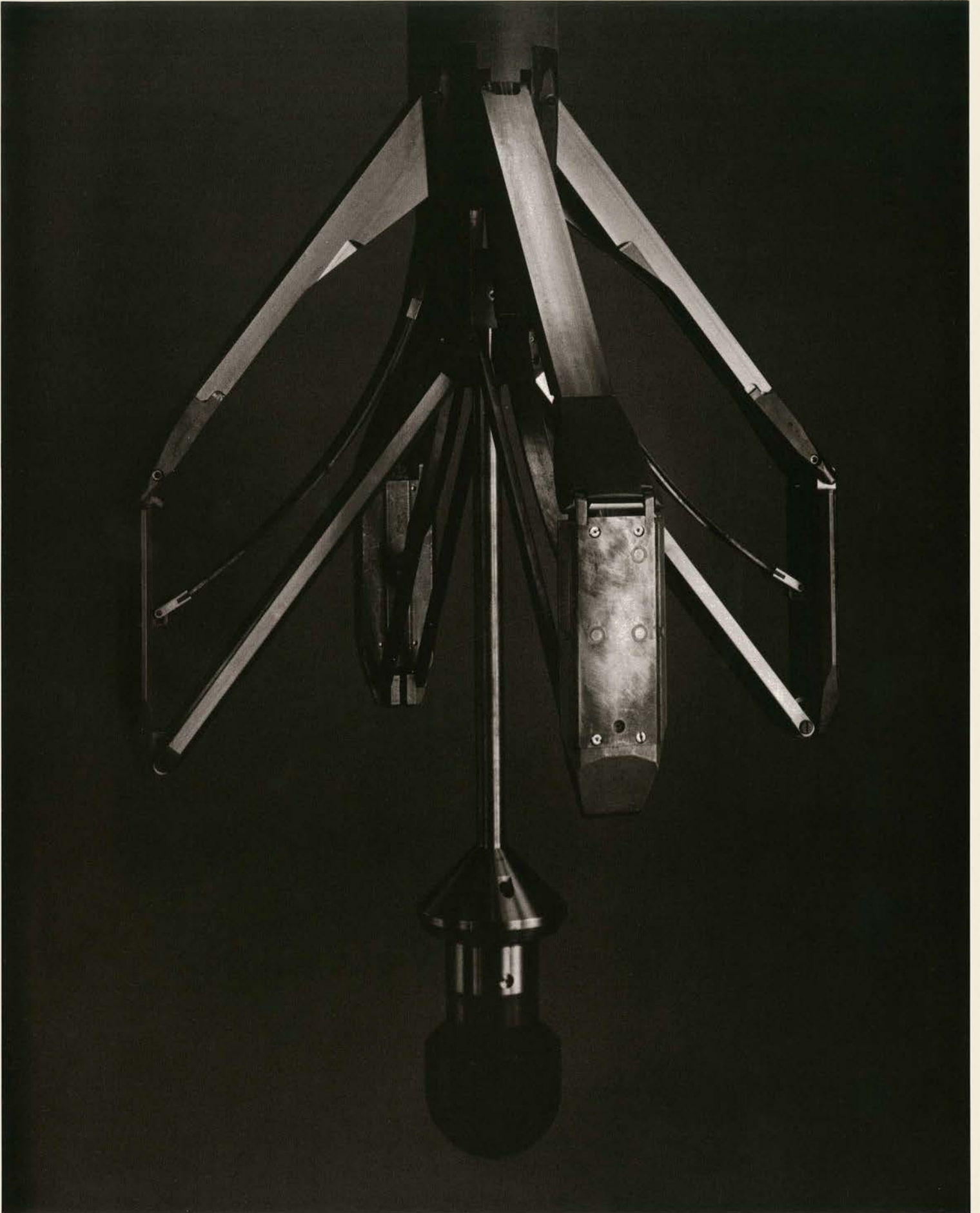
Four-armed stratigraphic high-resolution dipmeter measures the dip of formations penetrated by the well bore.
