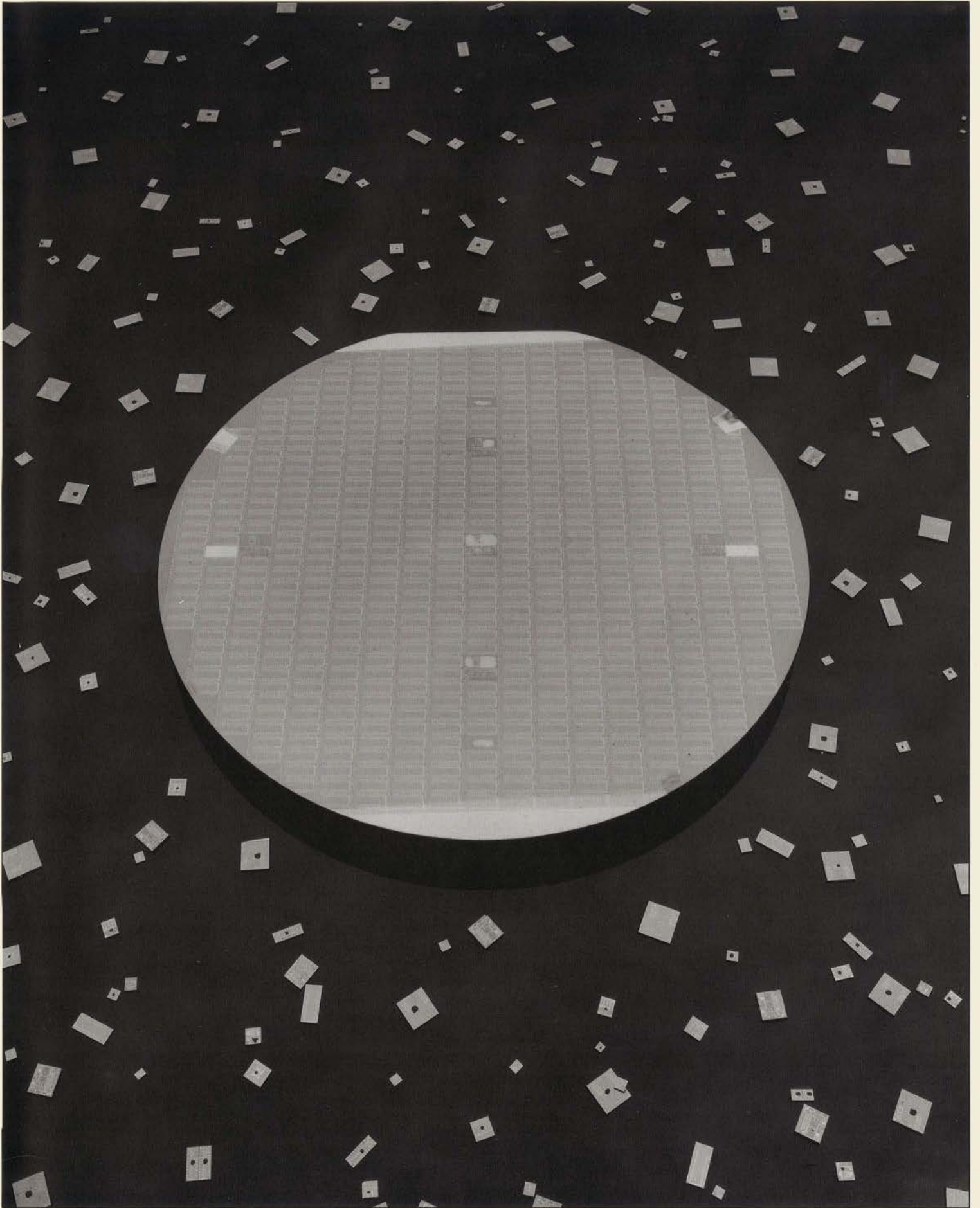
A processed silicon wafer (center) before it is cut into individual chips, surrounded by typical semiconductor integrated circuit chips.
