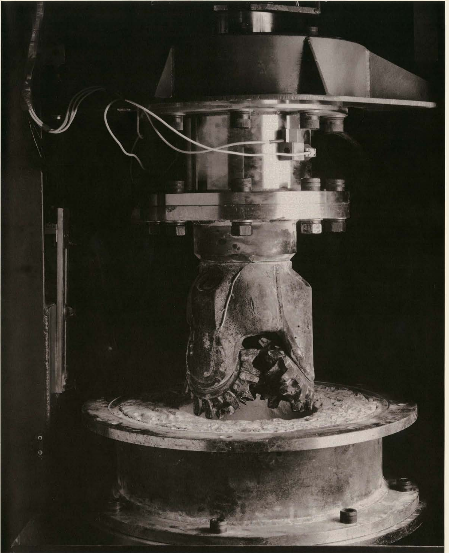
Experimental drilling machine at Cambridge Research. Measurements help determine the bit wear and the nature of the rock being penetrated.
