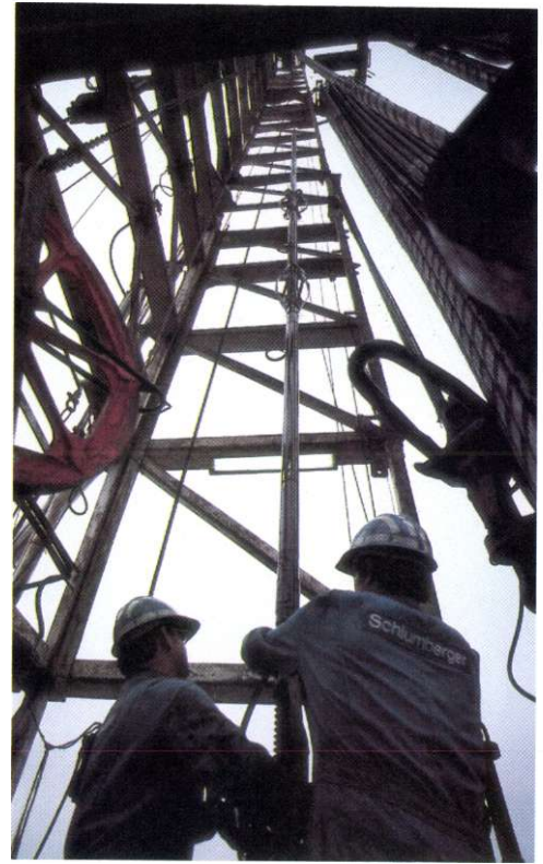
A Schlumberger crew prepares a combination tool for logging a well in the U.S. This tool permits three different wireline services to be run on a single trip in the well.
