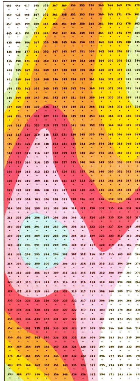
This map is one product of a Field Study. It shows reservoir parameters computed at each point of a grid covering the entire oilfield. In this example from Iran, the figures indicate the reservoir thickness in feet; the distance between two points of the grid represents 1000 feet. Colored contours delineate regions of constant reservoir thickness.
