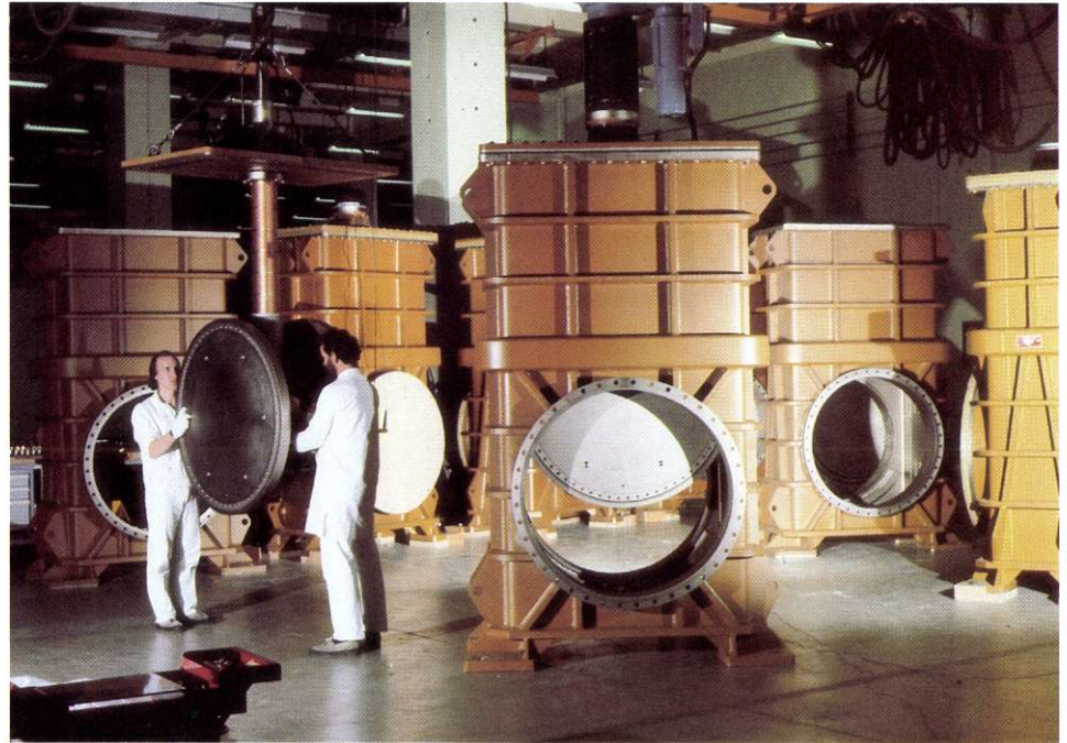
Assembly of nuclear valves to be installed in a uranium enrichment plant being built in France. This plant, the first of its kind in Europe, will produce uranium to fuel nuclear power stations.
