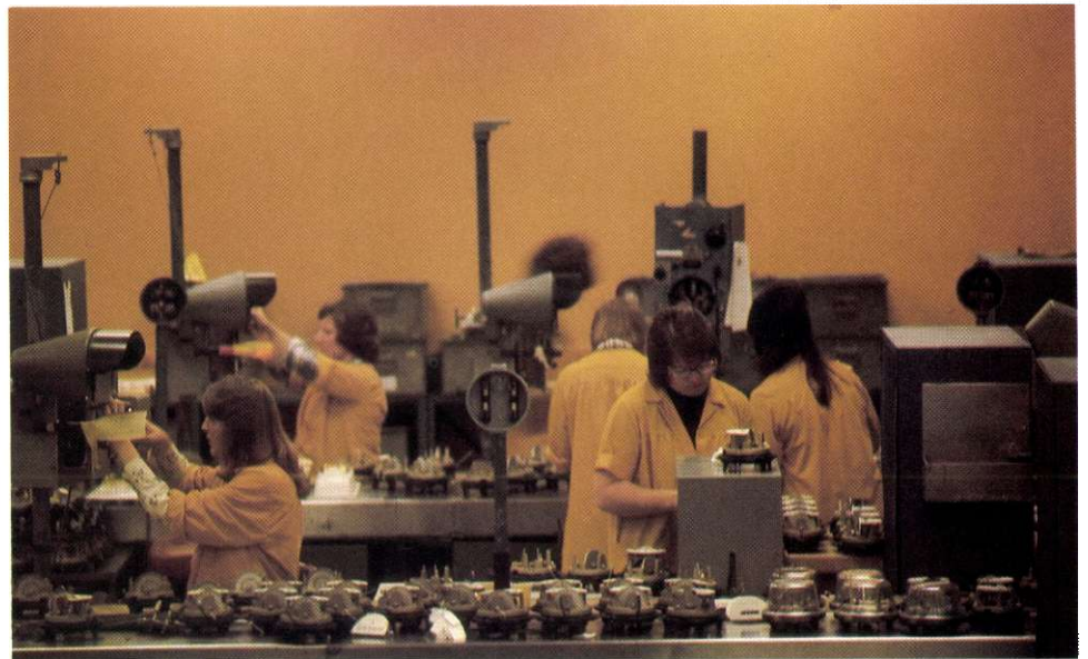
Part of the assembly line for residential singlephase watt-hour meters at the Energy Management division of Sangamo Weston in South Carolina.
