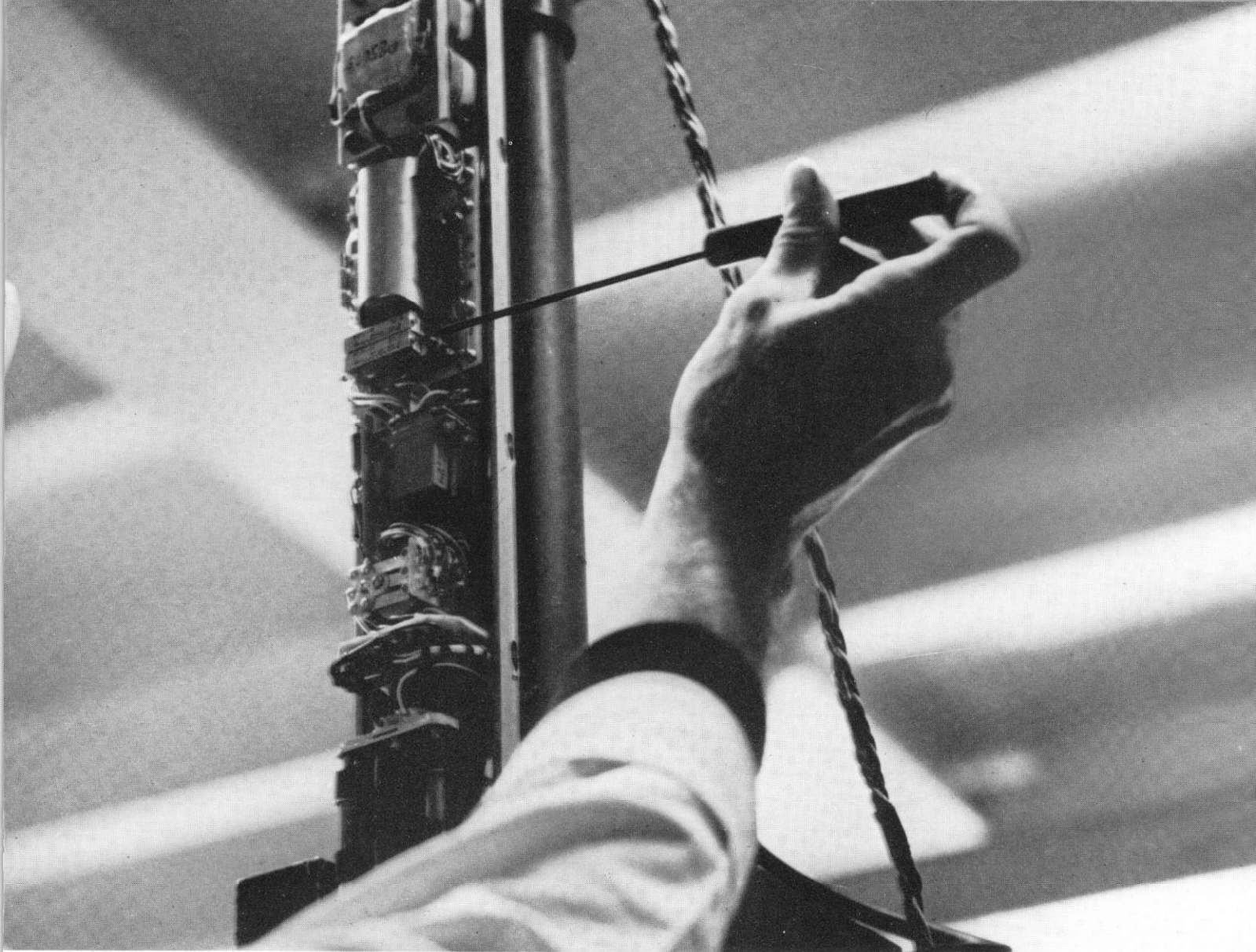
For precision measurement: a technician at our Paris engineering center calibrates an inclinometer for a dipmeter which measures the inclination from the horizontal of the formations intersected by the drill hole. These data assist in identifying underground geologic structures.
