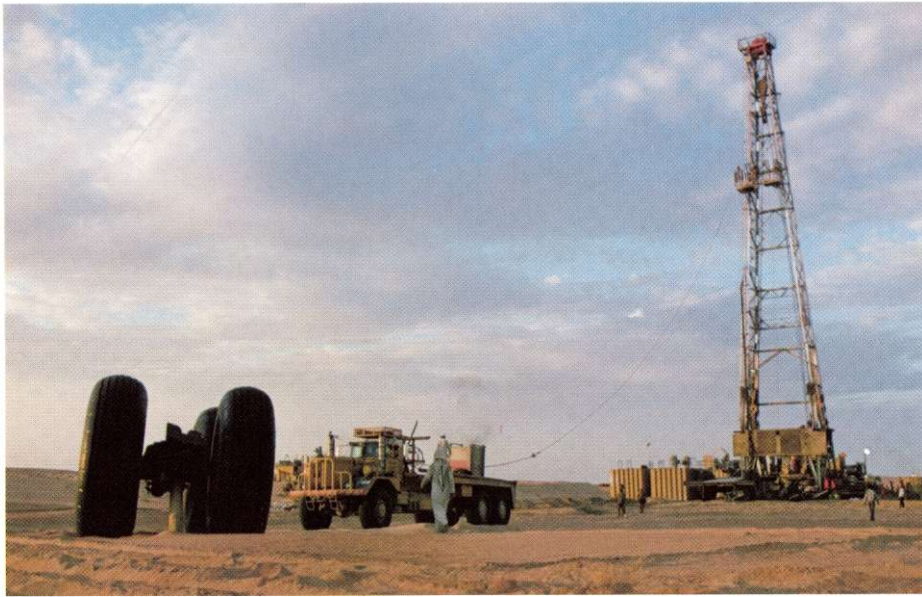
◀ A Forex Neptune rig in Anibawa, Nigeria, and the crew. A string of drill pipe is hanging from the derrick. Behind the men are four 475 HP engines that provide power for hoisting and drilling. The crew keeps this rig working around the clock. Most of them are Nigerian nationals including all of the drillers.
