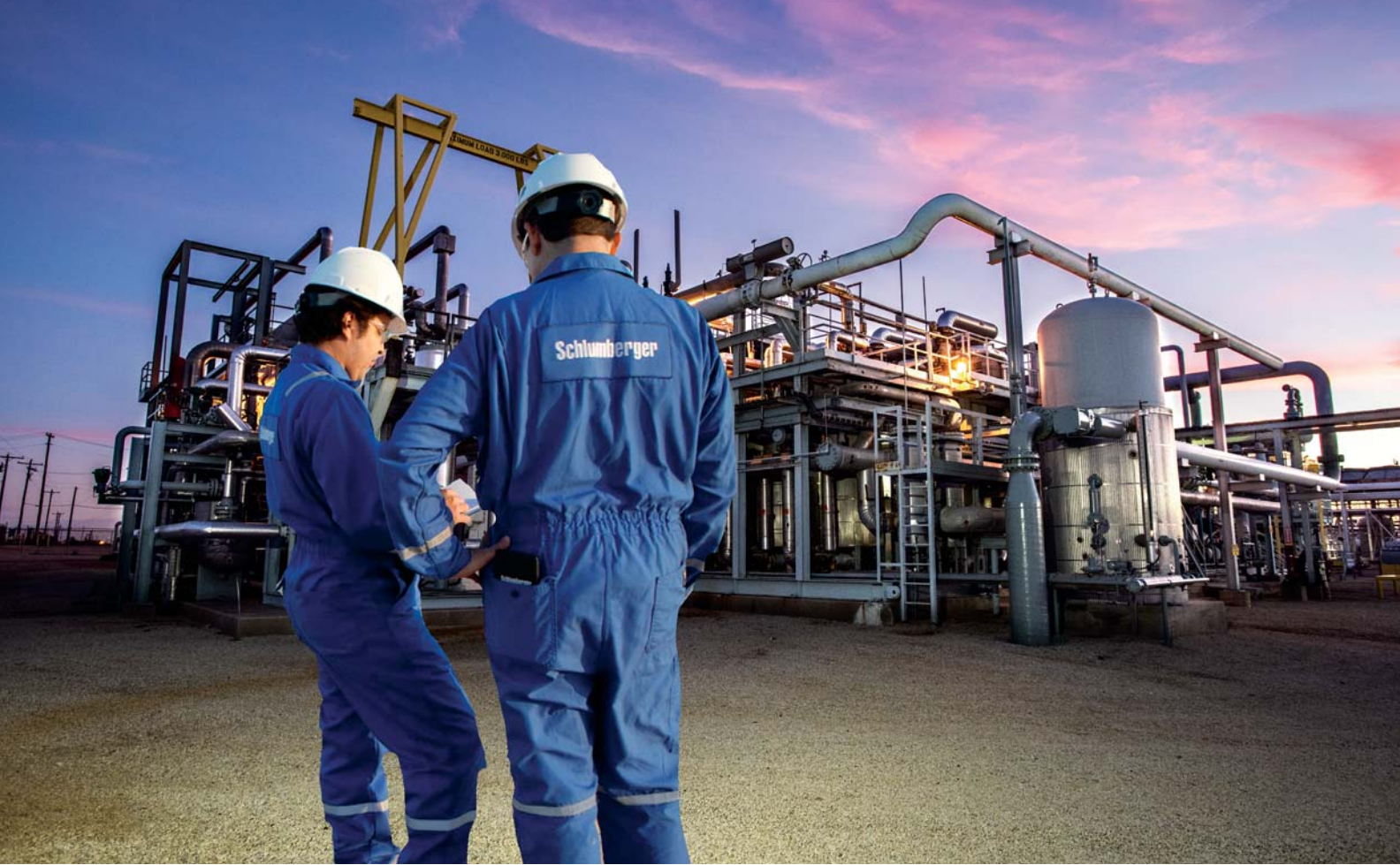
Process engineers review the performance of a land-based production system used to separate produced oil, gas, water, and solids. The oil is treated to meet sales specifications before delivery to the transportation system (i.e., the pipeline, truck, ship, or railroad car).
