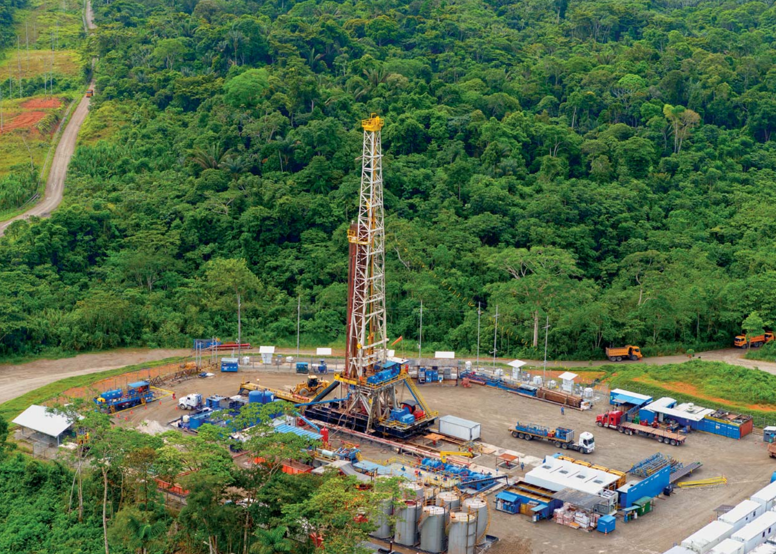
Schlumberger drilling and cementing equipment setup on a wellsite in Ecuador at the Shushufindi-Aguarico field ready to drill a horizontal well.
