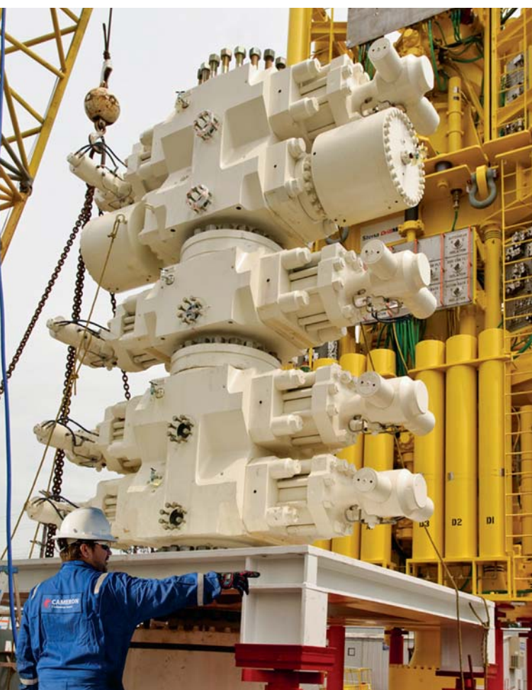
A drilling systems engineer prepares a five-cavity BOP stack and control pod for delivery to the customer.
