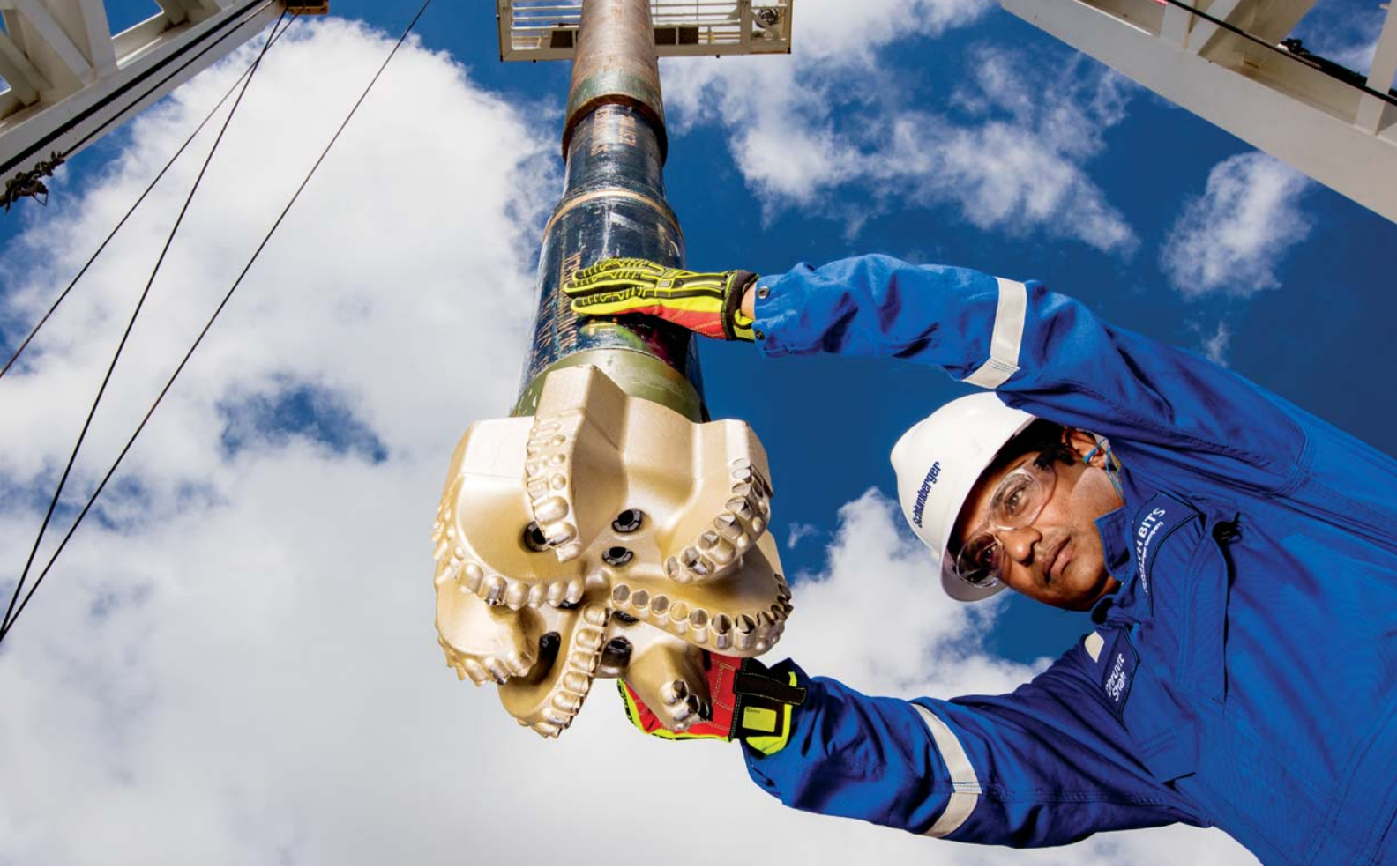
Mechanical Engineer Dhruvit Shah maneuvers a drillstring with an integrated bottomhole assembly and AxeBlade diamond element bit. AxeBlade bit technology employs a ridge-shaped geometry that cuts rock in a new way by combining the shearing action of a conventional polycrystalline diamond compact cutter with the crushing action of a tungsten carbide insert.
