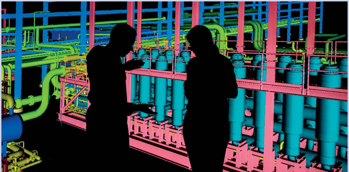
Engineers review a computer-aided-design image of the Scurry Area Canyon Reef Operators Committee (SACROC) gas processing facility for CO 2 reinjection and hydrocarbon recovery at the Digital Technology Theatre in Houston, Texas. This method of enhanced oil recovery frees the oil molecules from the reservoir's pores so they can flow into the production wells, where they are then separated in facilities such as the one shown here.
