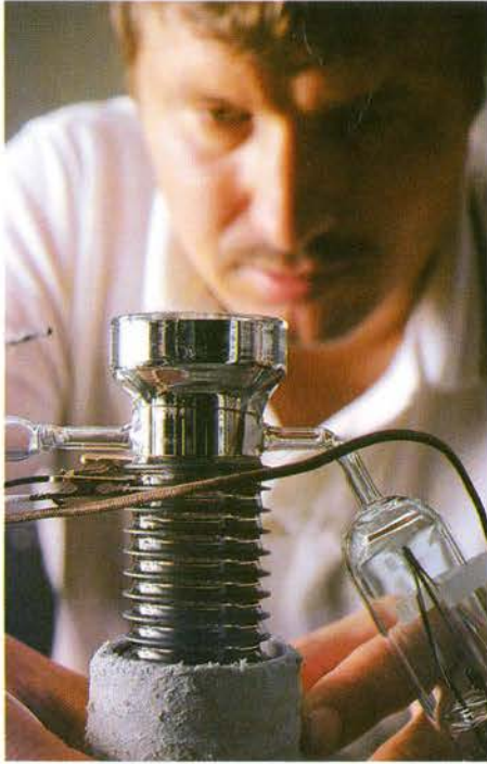
At EMR Photoelectric, fabrication of a high-temperature multiplier phototube used as a radiation detector in well logging.
