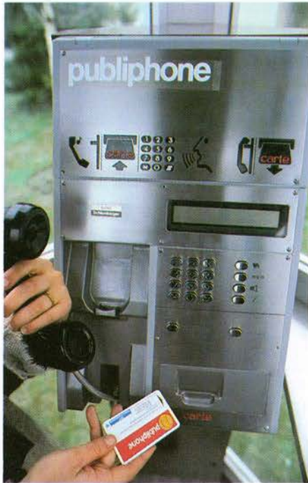
The new Flonic electronic payment card developed for use in public telephones.
