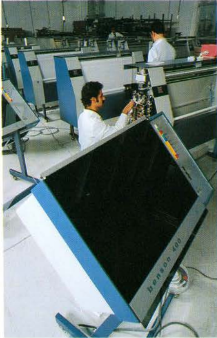
Benson plotters in final assembly and test in the Guérande, France manufacturing plant.
