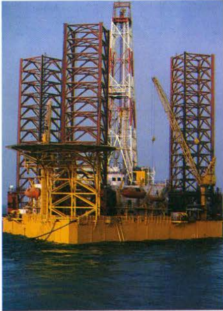
Trident III, an offshore jack-up drilling rig under tow to a new location.
