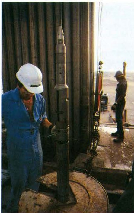
A Wireline engineer guides a logging tool being lowered in an oil well in the Middle East.
