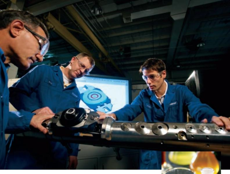
Once the technology was developed, it was crucial that it become commercially available as fast as possible. So rather than spending years developing a completely new tool to deploy the Quicksilver Probe technique, the Schlumberger engineering team leveraged our 50-year history of wireline formation tester design to engineer a solution that could be rapidly deployed on the fleet of formation tester tools already in service.
