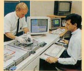
At the IBM plant in Corbeil, France, placing a wafer containing dozens of identical integrated-circuit chips on the wafer stage of an IDS 5000, in preparation for diagnostic tests.
