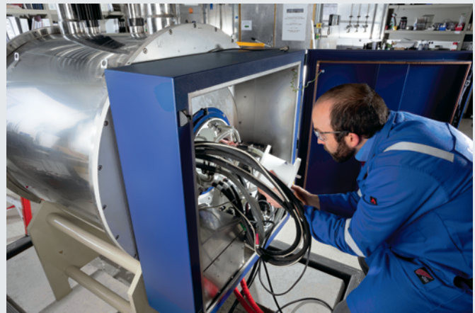
SDR Research Scientist Marcus Donaldson prepares to image a saturated reservoir rock sample in a high-field magnetic resonance apparatus. Magnetic resonance images provide information on rock porosity and permeability.
