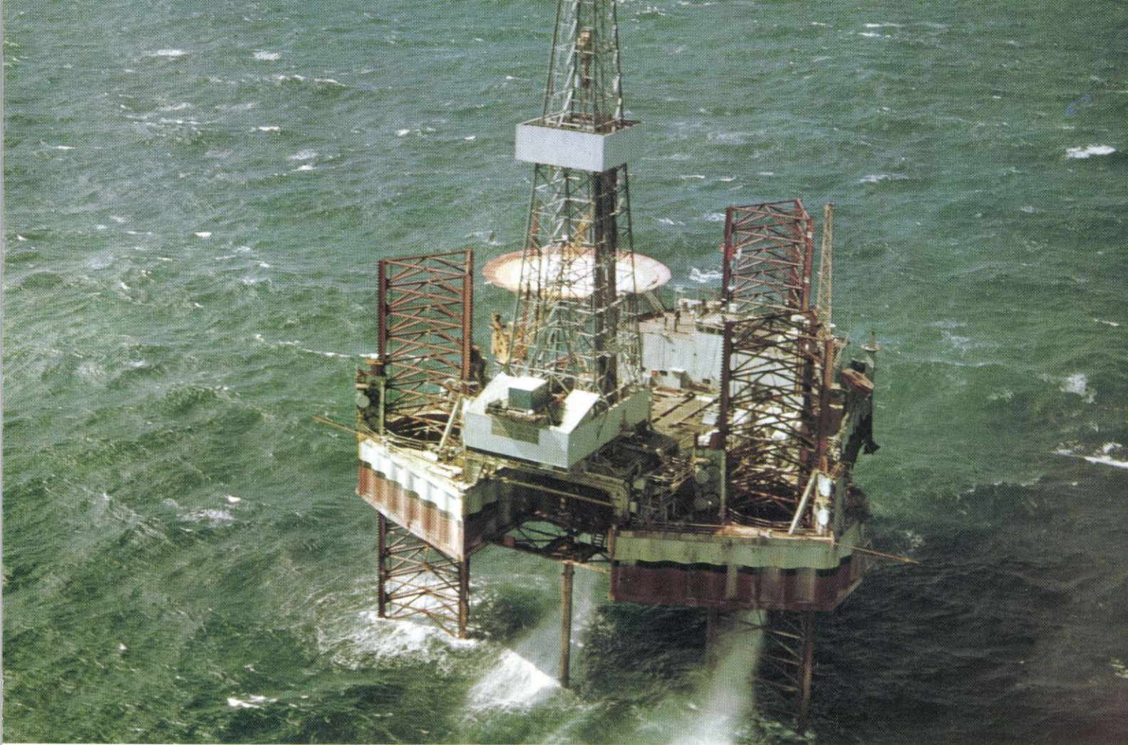
Neptune drilling platform in the North Sea. Schlumberger logging unit is in foreground.
