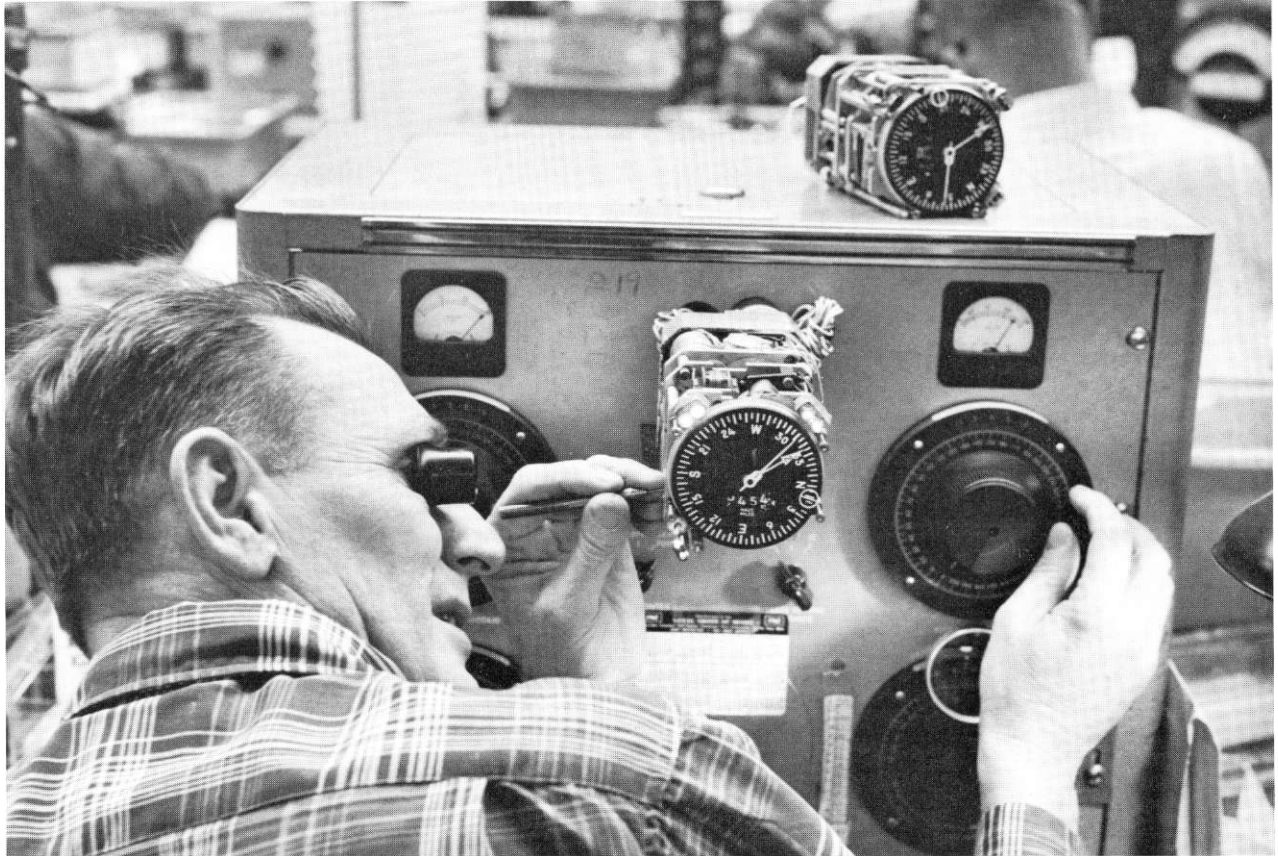
A wide range of aircraft measuring instruments is produced and inspected at the Newark, New Jersey, plant of Weston.
