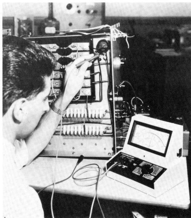
Above: Weston's new volt-ohm-milliammeter, the first portable of its kind to be packaged in a console-type case. Left: Launching of Apollo.
