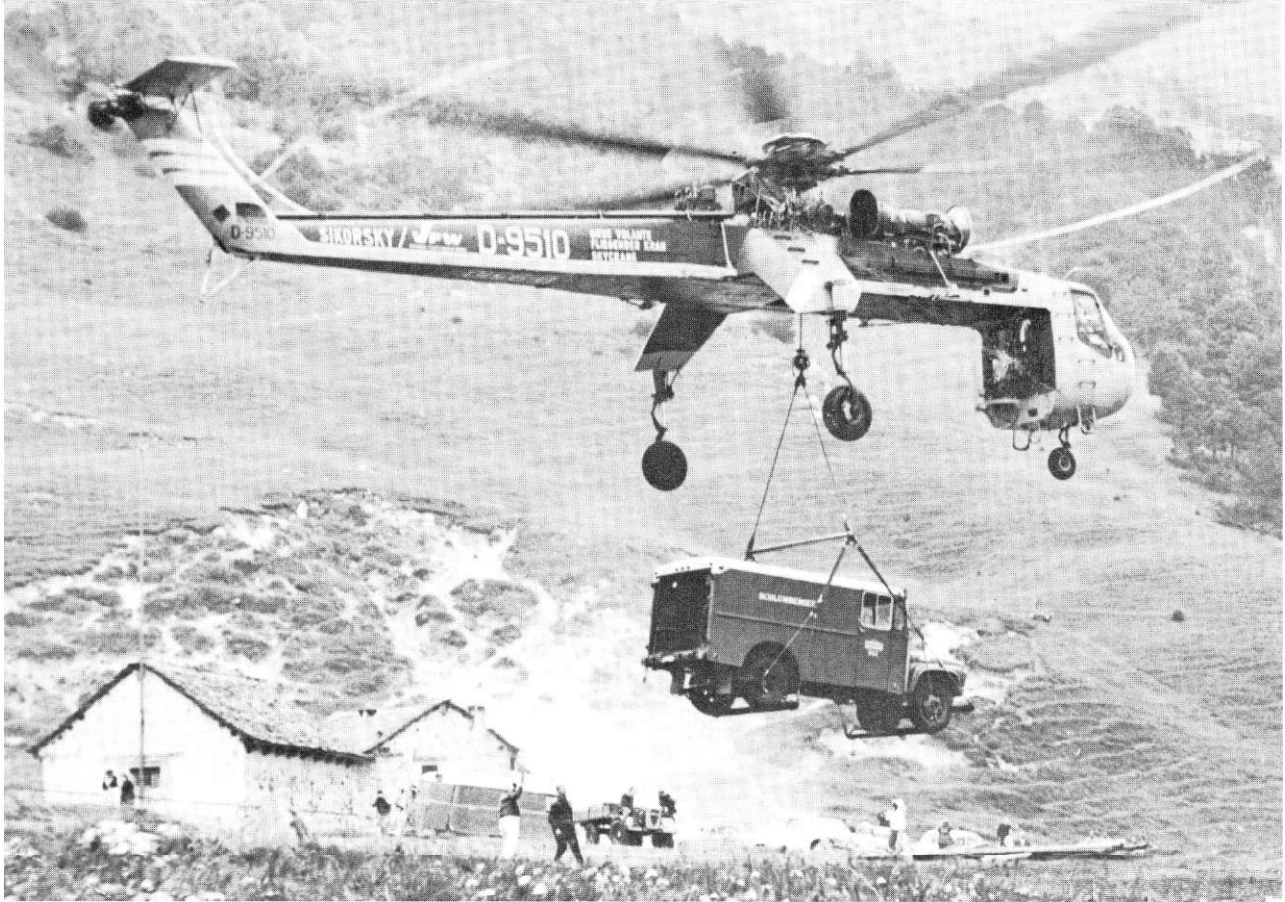
Schlumberger truck airlifted to survey geological conditions for a new Gothard tunnel in Switzerland.
