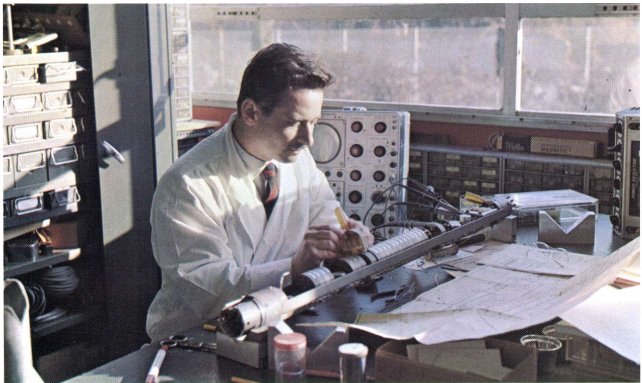
Checking a microsonic cartridge (Paris). Sonic logging is one of our 70 wireline services.
