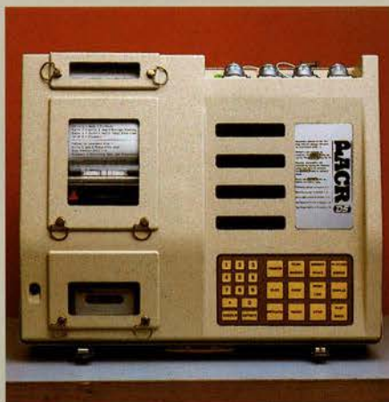
PACR (portable automatic cement recorder) is a rugged, on-site instrument for monitoring and recording data during cementing jobs.
