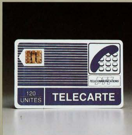
This smart card, with an embedded microcircuit chip, allows cardholders to pay for calls automatically on the new generation of French payphones.
