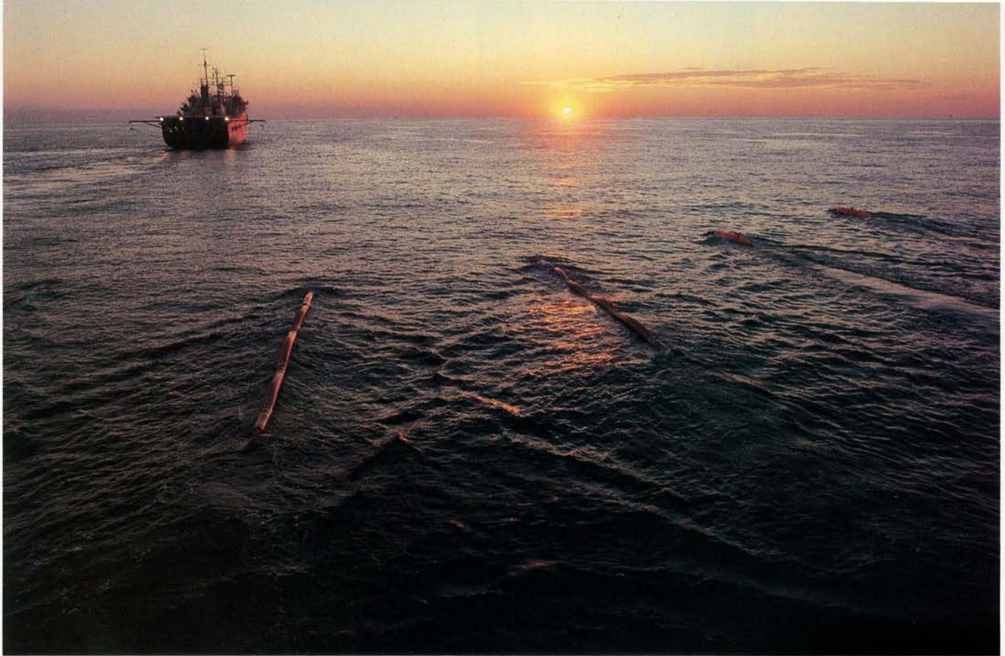
The GECO Searcher in the Gulf of Mexico towing multiple streamers used for 3D seismic surveys.
