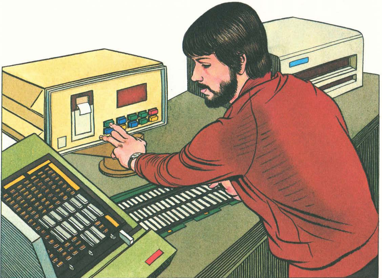
At a major computer manufacturer, a subassembly tester is automatically performing multiple tests on circuit boards.
